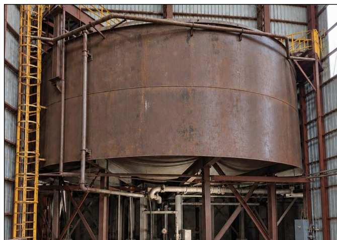
Figure 6: Industrial Thickeners at Site (Source: Company Documents)
